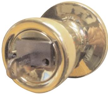
By drilling a small hole in the cylinder face, the retainer can be removed and the cylinder rekeyed easily. Replacement scalp plates are included with the tool and are easily replaced. Reinstall the retainer and spring, and the lock is back in working shape!
