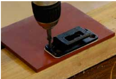
Step 25 - Install Strike to Frame Bracket
