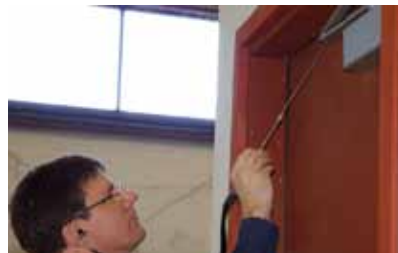
Step 29 - Check Gasket for Seal
