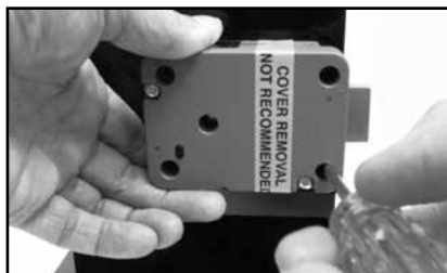
Figure 5 - Tighten Mounting Screws
