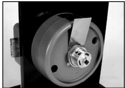
Figure 20 - Place Gauge Between Dial Hub & Bushing
